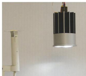
LED thermal test configuration
